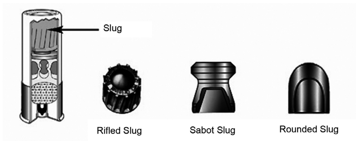
Figure 14. Types of shotgun slugs
